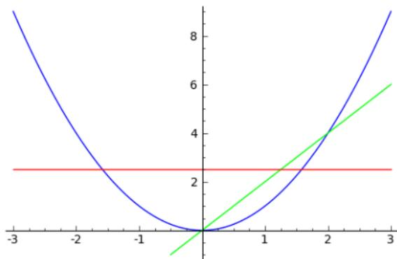
The blue drawing is the graph of our function. The green secant line is our average rate of change over the interval  $[0, 2]$ . The red secant line is the average rate of change over
